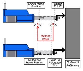
Fine tuning the position can be done using the same manual handle after pressing
