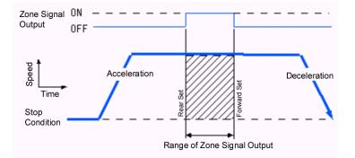
If you activate the extended functionality, you can set the ZONE signal output range individually for each Position with using "Individually settable ZONE signal output range for each Position" extension. You can make the mechatronics cylinder to check the stopped position is regular or not, even if the target works have many kind of length.
