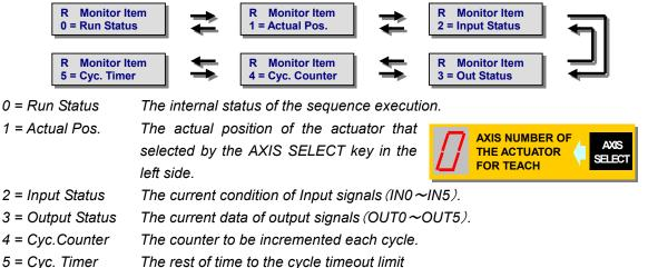
The cycle counter is reset to 0 when CTC-33 is powering ON, and it's incremented by 1 at the end of in every sequence execution cycles. So the value of the cycle counter is always same as the total number of sequence cvcles after powering ON.
